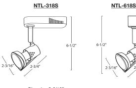
Diameter: 2-3/16" Length: 2-3/4" Max. Extension: 6-1/2" Transformer (NTL-318S): 4-3/8"L x 1-3/8"W x 7/8"H
