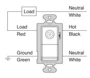
The WN-100 can be wired for singlelevel lighting (shown), or for manual bi-level control.
