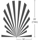
— 10'— (3.1m) The WN-100 has a coverage range of 180° and a maximum coverage area of 300 ft<sup>2</sup>. To maintain its coverage capacity and optimally detect motion, the WN-100 must have a clear and unobstructed view of occupants.
