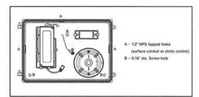
Prepare the back-plate for mounting by drilling out the two corner and the center 5/16" diameter holes ("B").
