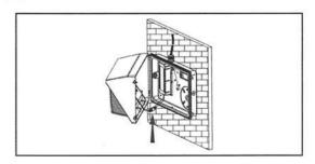
9. Fasten the front housing assembly to the back plate.
