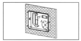
If wiring is performed using a recessed junction box then drill out the appropriate junction box holes.
